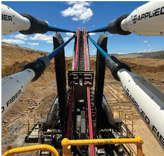
Figure 2. Shock damping fibre pendants on 4100 Shovel.
