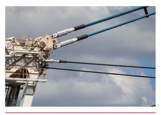
**Figure 2.** Applied Fiber Bridon Tiger Blue Pendants – showing main and intermediate boom support pendants connecting at tri structure on dragline.
