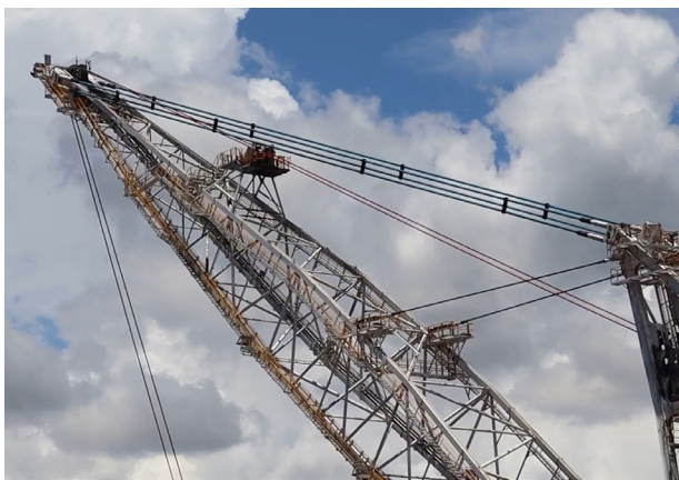
Figure 3. Fibre pendants running on a Marion 8050 dragline.
