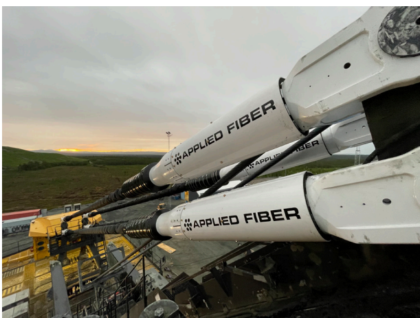
Figure 5. Shock damping fibre pendants installed on P&H 4100 C Electric Rope Shovel.
