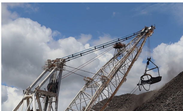
Figure 4. Dragline operating is smoother with fibre main pendants.
